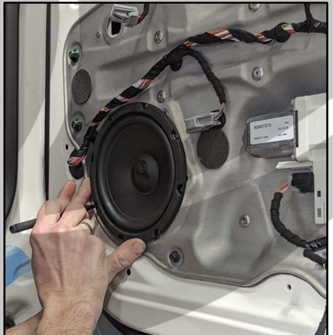
20. Mark drill holes for the next step
