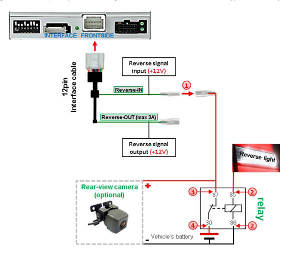
① Disconnect the green cable's preconnected male- and female connectors of the 12pin interface cable and connect the green input cable "Reverse-IN" to the output connector (87) of the relay.
