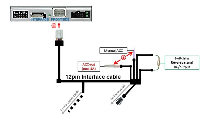
1 Connect the red wire ACC-OUT and the purple coloured wire Manual ACC of the 12pin interface cable to +12V ACC power supply.
