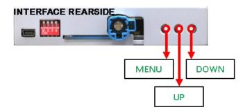
The picture settings are adjustable by the 3 push-buttons at the rear-side of the video-interface. Press the MENU button to open the OSD settings menu or to switch to the next menu item. Press UP and DOWN to change the selected value. The buttons are placed inside in the housing to avoid accidental changes during or after the installation. Picture settings must be done separately for all video inputs while the corresponding input is selected and visible on the monitor.
