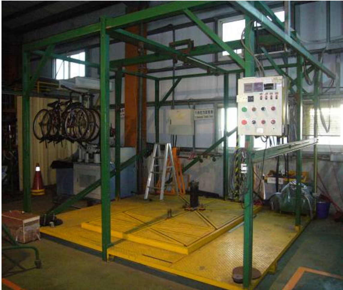
Figure 1 - Six Dimension Tensile Test
