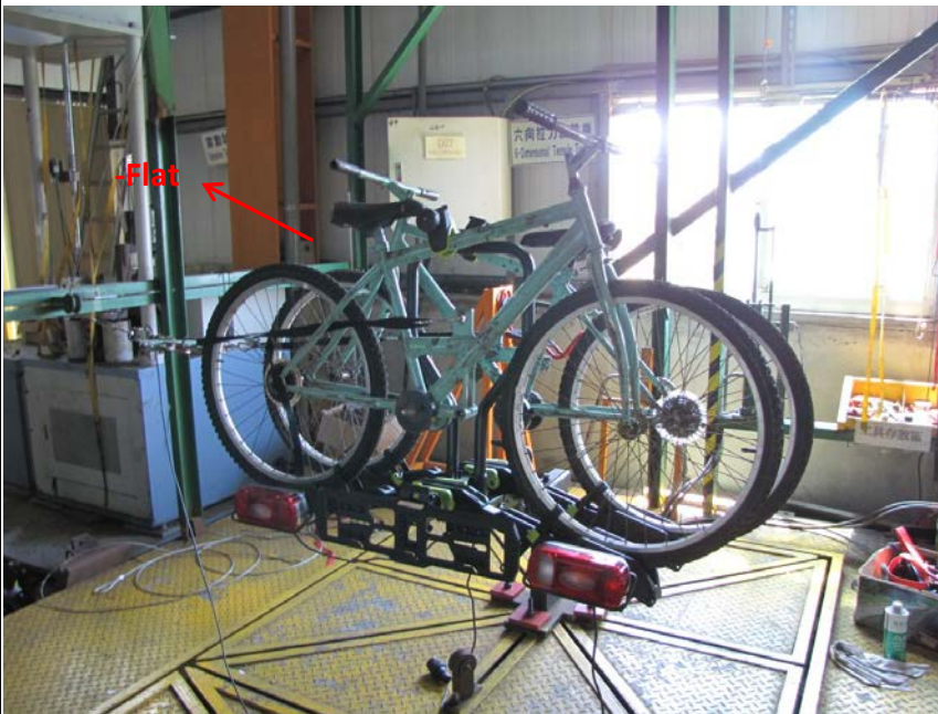
Figure 14 - -Flat test, Force=162kg.
