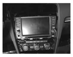
Carefully unclip the original panel, remove from it and save the air vents and the silver frame.
