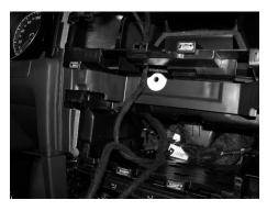
Remove the OEM head unit using Becker keys.
