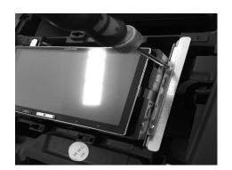
Connect all cables, insert the AFT unit into the housing and fix it with the supplied screws as show in the picture.
