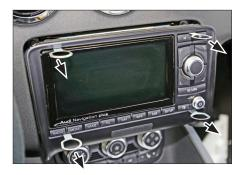
1. Remove OEM head unit with radio release keys
