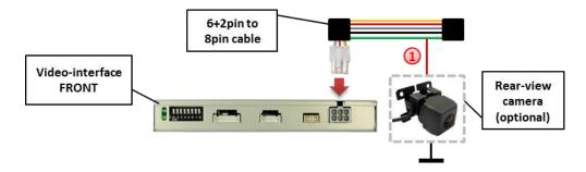
1 Additionally, the +12V (max. 500mA) power supply for the rear-view camera can be taken from the green wire of the 6pin to 8pin cable.
