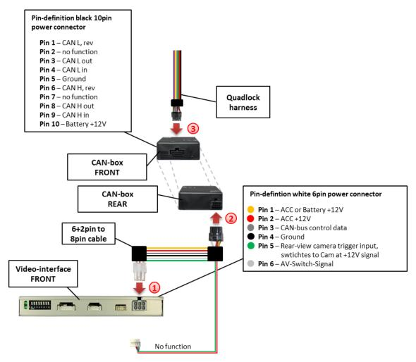
1 Connect black female 10pin Micro-Fit connector of the Quadlock harness to the male 10pin Micro-Fit connector of the CAN-box.
