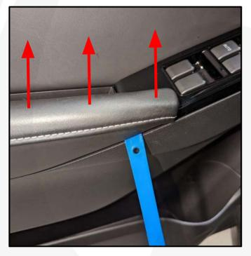
15. Remove the window switch panel
