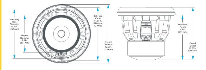
Net volumes given below do not include the air volume displaced by the speaker (Driver Displacement). This value must be added to the net volume along with the displacement of any braces and/or ports (if applicable) to arrive at a gross internal volume. Air inside a port is not part of the effective net volume. Calculate ports as solid, not hollow objects.
