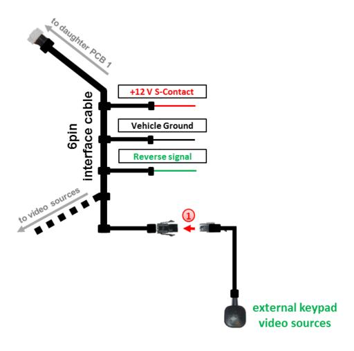
1 Connect the keypad's female 4pin connector to the male 4pin connector of the 6pin interface cable.
