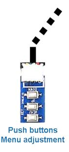
The picture settings are adjustable by the 3 push-buttons of the daughjter PCB's menu keypad. Press the 1. button to open the OSD settings menu or to switch to the next menu item. By pressing the other both push buttons the selected value will be changed. To avoid accidental changes during or after the installation, we recommend to disconnect the keypad from the pushbutton cable after the adjustments are done. Adjustments have to be done, while the selected input is visible on the monitor.
