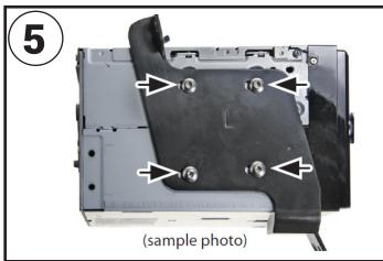
Mount the left and right brackets to the head unit using the supplied hex screws.
