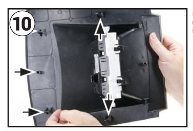
Remove the five clips from the original fascia panel and replace them onto the new display panel as shown in the image.
