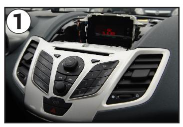
Use a panel removal tool to unclip the panel surrounding the small dash display. Remove the entire trim panel and place safely to one side for reassembly.
