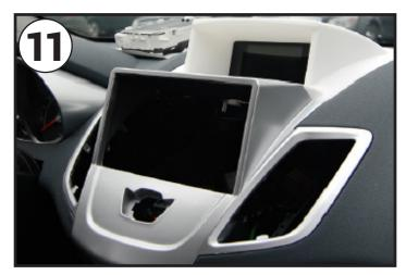
Make all required wiring connections to the back of the aftermarket head unit and fit the head unit/fascia/display assembly into the dashboard cavity to complete the installation.
