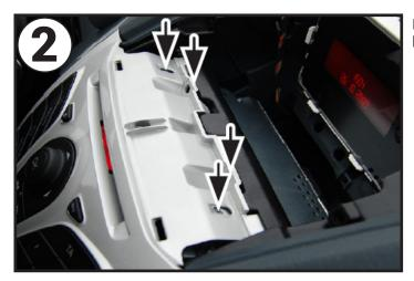
Remove the four screws highlighted by the arrows located above the OEM head unit.
