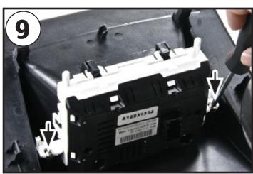
Fix the display into position using two supplied screws at the points highlighted by the arrows in the image.
