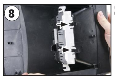
Push the bottom of the OEM display until it snaps into place.
