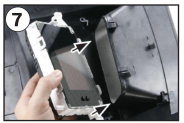
Mount the OEM display to the display panel by turning the panel upside down and placing the display as shown in the image.
