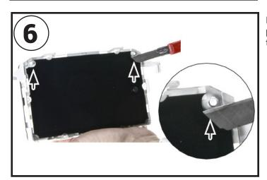
Remove the OEM display and cut away the overlapping pins on the left and right as highlighted by the arrows in the image.
