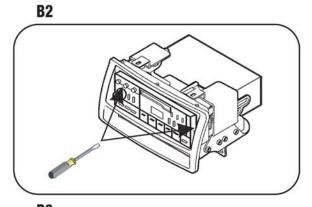
Re-connect the battery terminal and test the unit for proper operation. Snap the factory head unit trim bezel over the kit by engaging the (4) bracket tabs ("A") and (3) Housing bosses ("B") to the back of the bezel. Slide the assembly into the subdash and mount with (4) 10 mm bolts previously removed in step #1. Re-assemble the dash. (See Fig. B3)
