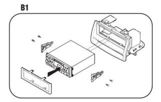
NOTE: To remove the mounted head unit, unclip and remove the ISO Trimplate.
