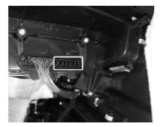
7. Connect the 8-Way connector to the MOST Interface
