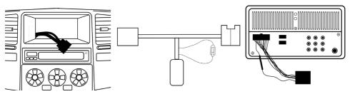
\*Connect required analogue flying wires to aftermarket head unit using colour table.
