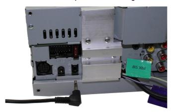
4. Connect the 14 way molex connector to the interface.
