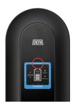
Locate the Charger ID referencing to the installation/group. The ID is found on the front of the charging box.
