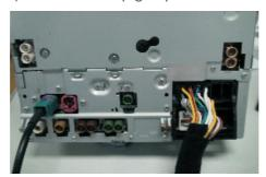
3. Plug the original grey LVDS connector removed in step 2, into the green LVDS connector on the interface. Connect the white 5 way connector from the other end of the supplied LVDS cable (Fig 1, 4) to the interface. Connect the black 8 way connector of the vehicle power T-harness (Fig 1, 2) to the interface.
